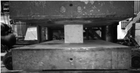
图4 立方体抗压强度加载设备 Fig. 4 The loading equipment for testing cube compressive strength
