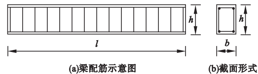
图 1 PVA-ECC-钢筋复合梁示意图 Fig. 1 Schematic diagram of PVA-ECC-reinforced composite beam
