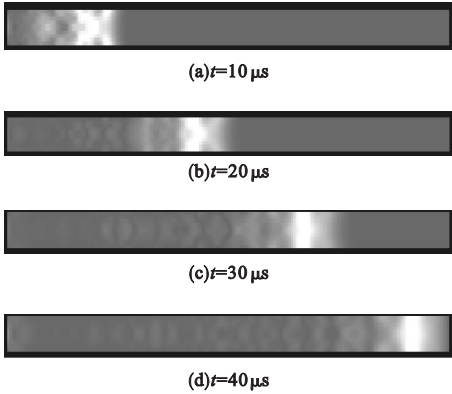
图 5 模型 II 应力波在自由端反射之前传播过程 Fig. 5 Propagation process of stress waves before reflection at the free end of model II
