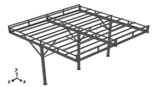
图1 新型装配式临时作业棚结构形式 Fig.1 Structural form of new prefabricated temporary work shed
