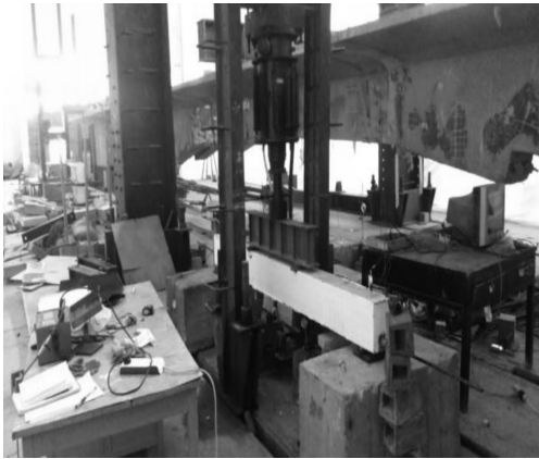
图7 疲劳试验装置 Fig. 7 The field fatigue test equipment
