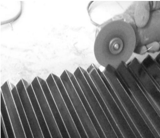
图4 波纹吸热板 Fig.4 Corrugated heat collector
