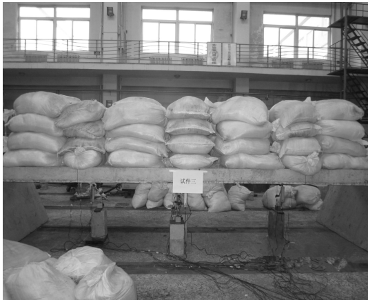
图3 预应力带肋叠合板加载 Fig. 3 Prestressed ribbed composite slab loaded
