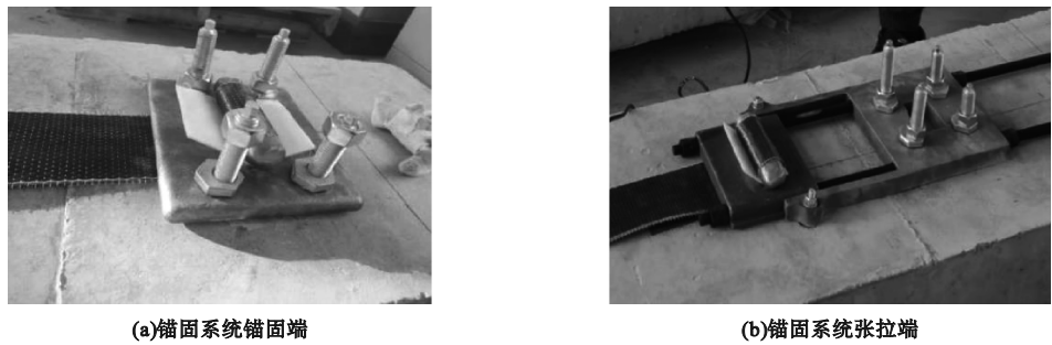
图1 穿孔式自锁锚具 Fig. 1 Perforated self-locking anchor system
