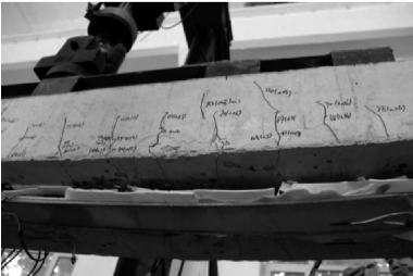
图9 试件CS2加载形态
