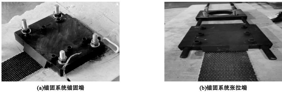
图2 模腔式自锁锚具 Fig. 2 Mold cavity self-locking anchor system
