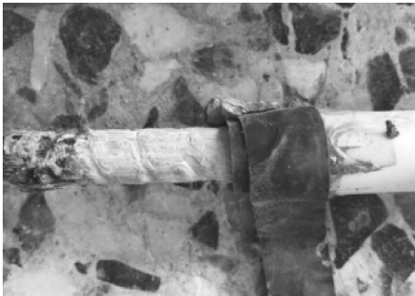
(a)GFRP筋肋剪切破坏
