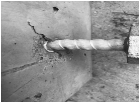
(c)局部混凝土劈裂破坏
