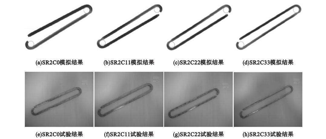
图7 有限元模型与试验试件的最终破坏形态 Fig. 7 Failure modes of finite element model and specimens
