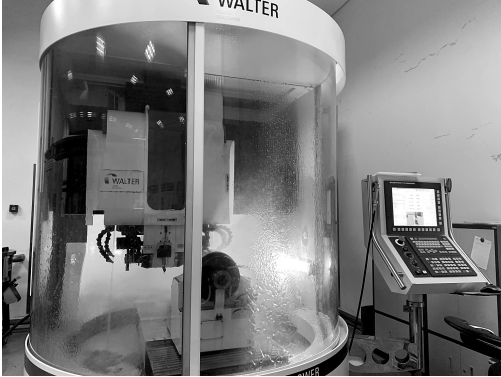
图1 数控工具磨床 Fig.1 CNC tool grinding machine
